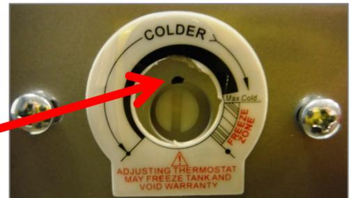
Turning the adjustment screw clockwise to lower the set point temperature.
